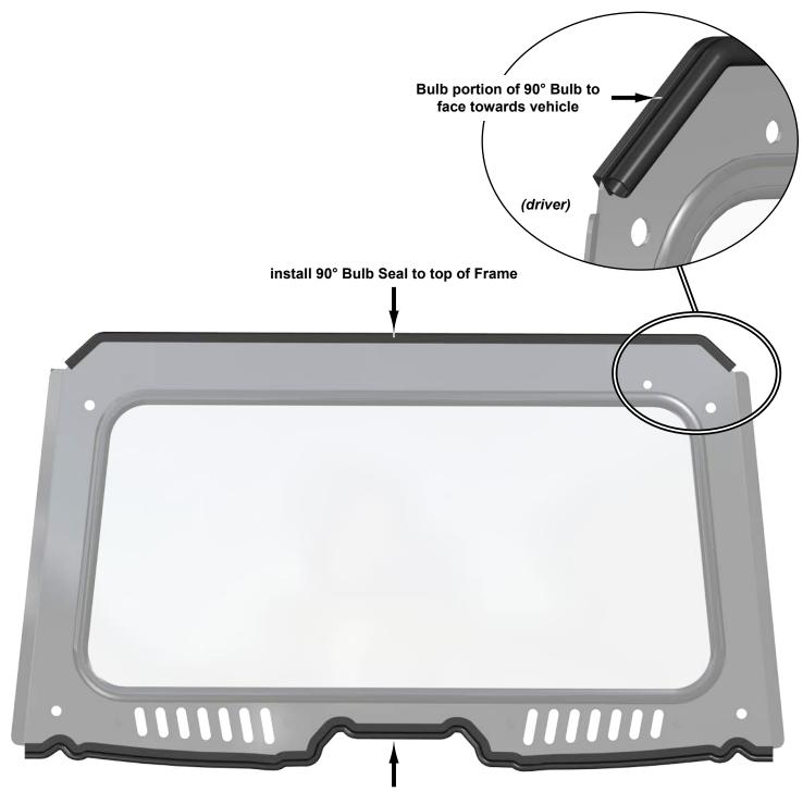
install Bulb Seal to bottom of Frame
