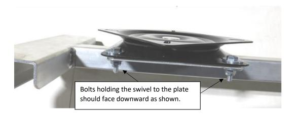
3. Place seat bottom up and align the swivel slots with the threaded inserts in the seat bottom. Secure with the Philips head machine screws and washers at all four corners.
