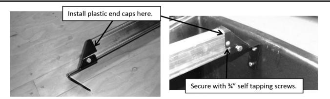
6. After the brackets and end caps are installed, the seat rail may be bolted into place with the 1/4" bolts, washers and nylock nuts using the previously drilled holes. Install plastic base and seat onto the rail. Use WD-40 or silicone to lubricate plastic seat base opening so it will go onto the aluminum rail easier.
