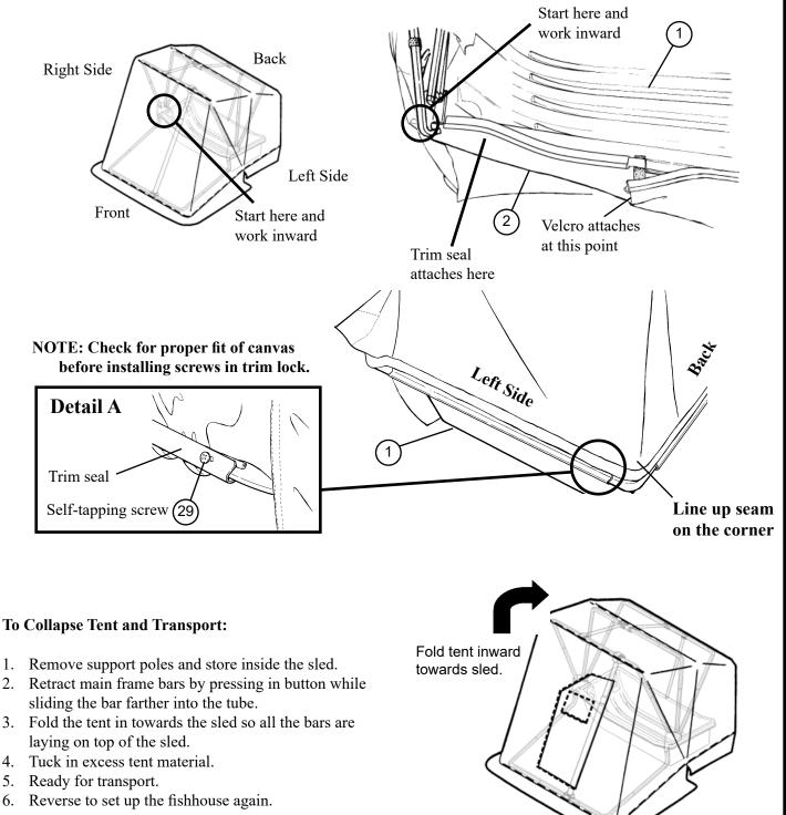
General Note: Be careful with tent windows in cold weather, as creasing or crushing them will cause breakage.
