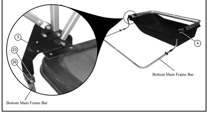
19. Set up main frame bars by grasping with both hands and pushing upward until button clicks into place. Start with bottom main frame bar and continue to the back main frame bar pushing lengthened bars into appropriate position.
