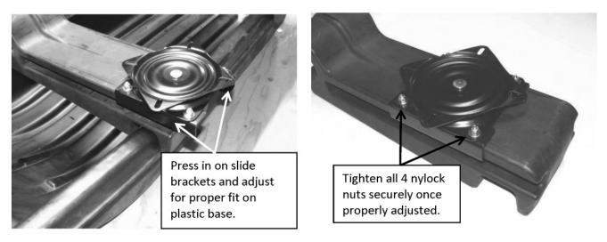
3. Line up the swivel with the inserts in the bottom of the seat. Loosely install the 1/4" x 3/4" phillips head bolt with washers (included in the seat box) into the inserts in the bottom of the seat. Tighten all 4 bolts securely once the swivel is properly positioned.
