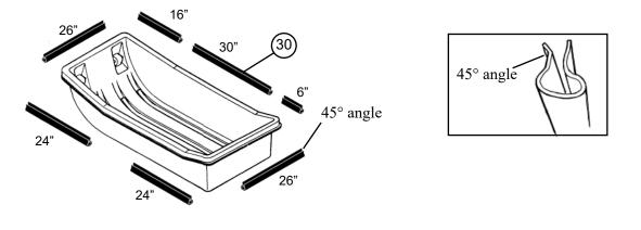
23. On the front of the fishhouse, start in the corners and work inward, snap the plastic trim seal on the canvas tent (Item 2) to the **lip** edge of the sled (Item 1). The tent (Item 2) will meet in the middle and should be free to open and close so it can be removed.
