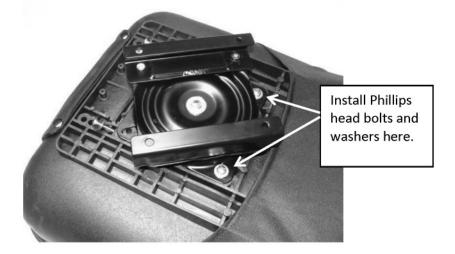
4. Drill out the four pre-marked holes for the seat rail brackets as shown using a 5/16" drill bit. The sled may be tipped upside down to make drilling the holes easier.
