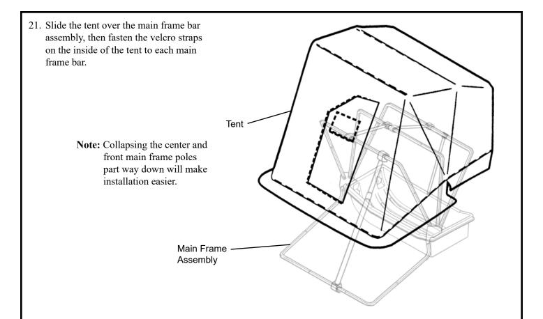
22. Once the canvas is on the frame and the Velcro attached, extend all of the frame bars upward and make sure all of the support poles are installed. Extend the front adjustable support pole so that the fabric in front is snug and not sagging. It will be necessary to loosen the back adjustable pole to achieve this. Once the front is set and the top support poles are in place, the back adjustable pole can be extended until it is snug. Install the plastic trim lock in the positions shown below.
