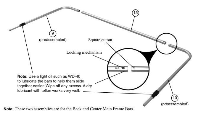
12. Position middle main frame (Item 15), left side front elbow and extension (Item 11), and right side front elbow and extension (Item 12) as shown. Align locking mechanism in item 15 with square cutout in items 11 and 12 and slide together until they lock. Lubricate frame bars for best operation as shown in step 11.
