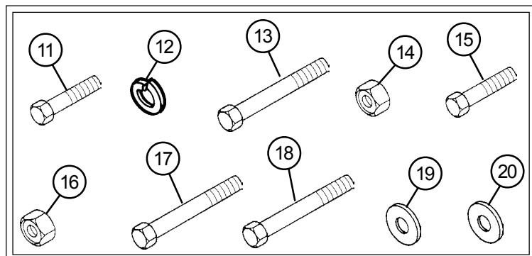
1. Attach the axle (Item 2) to the bottom side of the trailer (Item 1) with 7/16 x 1 bolts (Item 11) and 7/16 lock washer (Item 12).
